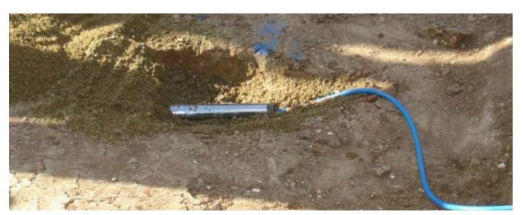
Vibrating wire piezometer in embankment dam foundation
