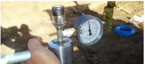
Saturation of HAE filter with saturation device
